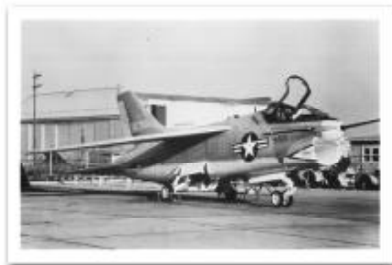
The first A-7A with an 11,350 lb thrust Pratt and Whitney engine flew in September 1965. The last of 850 A-7s were retired from the Navy's inventory following participation in Desert Storm combat operations.
