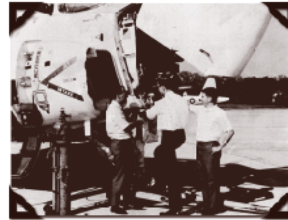
Testing of a Norton phased array antenna installed in an A-6A airplane, 1968
